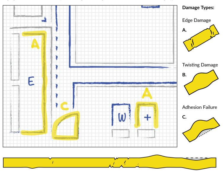
Tape with little to no damage can safely remain installed.
