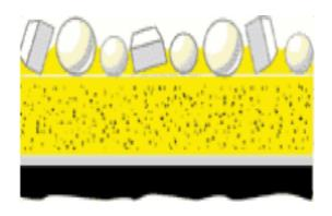
Removable Road Marking Tape offers excellent daytime visibility for delineation and superior nighttime reflectivity. The pre-applied, pressure-sensitive adhesive extends the application season typically shortened by marginal weather conditions. Quick and easy installation: simply prepare the surface, apply the tape, and tamp in place. When the job is completed the reinforced fabric backing makes removal easy. Marked roadways can be opened to traffic immediately.
