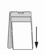
Slide through, pulling sign in front of bottom slot until sign hits the ground
