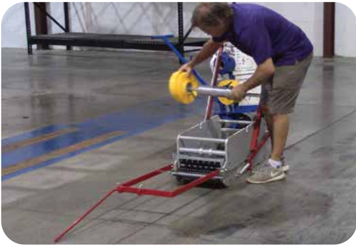
Step 3: Load a roll of Superior Mark® Floor Marking Tape on to the Tape Dispenser Roll (B).
