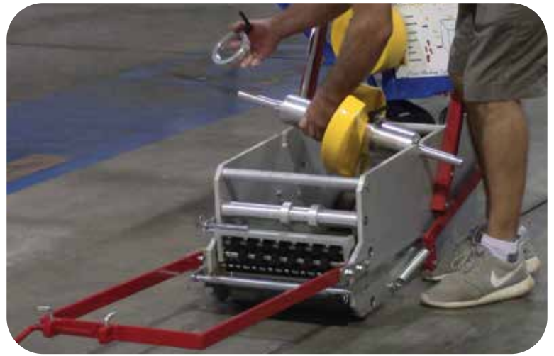
Step 4: Replace Tape Ring (C) and reset Tape Dispenser Roll (B) back into place.
