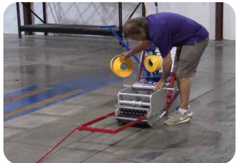
Step 2: Lift Tape Dispenser (B) and remove Tape Dispenser Ring (C).
