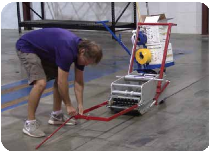
Step 1: Lay down guiding rod system (A).
